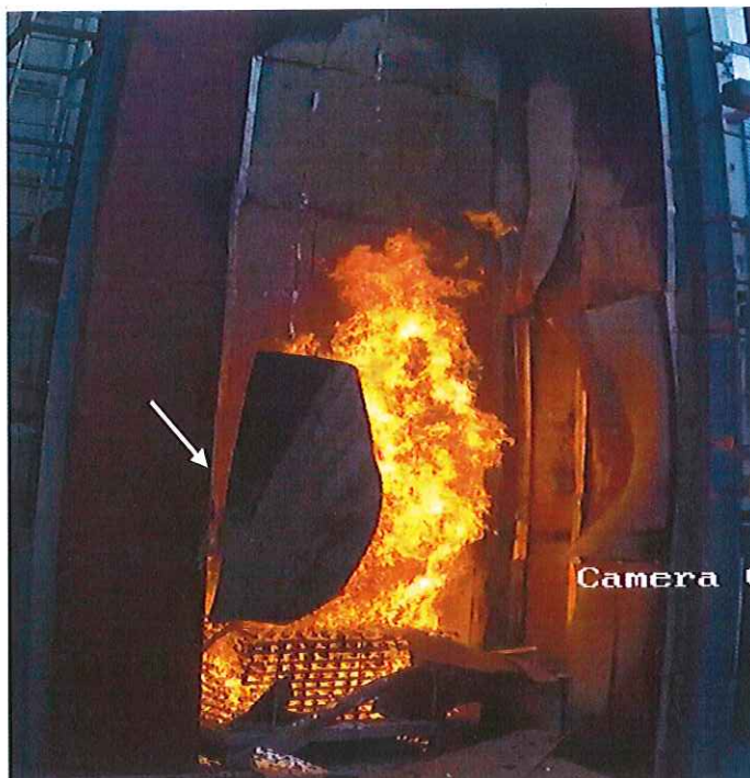
DLP C2858/0009 Panel M8 detached and fell off the main wall.
